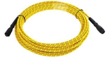
Prosino sensing cables detect the presence of water at any point along their length. Installed with a prosino locating module(P-LFP1), the cable senses water intrusion, triggers an alarm, and pinpoints the location.
